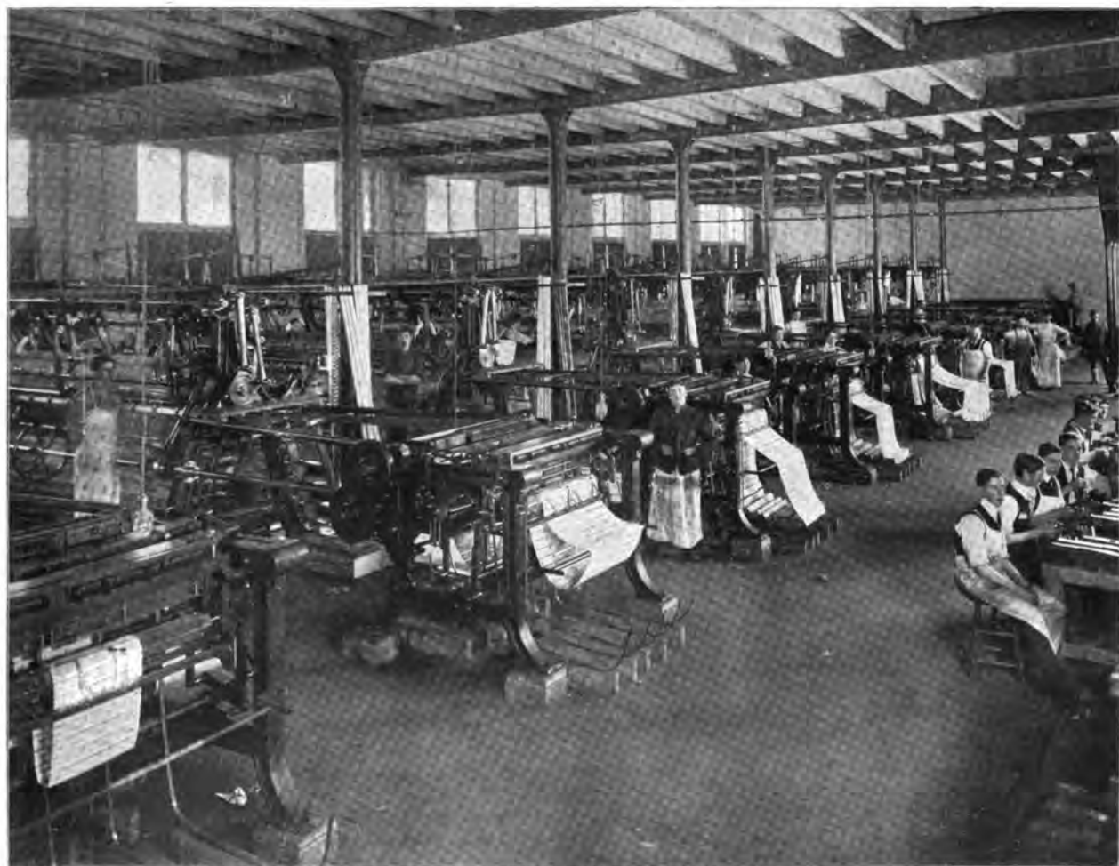
Portion of Zion Lace Industries, Interior View, Showing Levers Lace Machines
